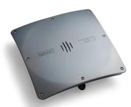
The XT-5 "all-in-one" RFID UHF Reader, with an integrated circular, polarized antenna and controller, is prepared for outdoor use in all weather conditions. It is ideal for applications in demanding environments that require a more cost effective Reader and Tag solution. Built around a standard Linux operating system, this Reader allows for in-house customization to specific project needs.
